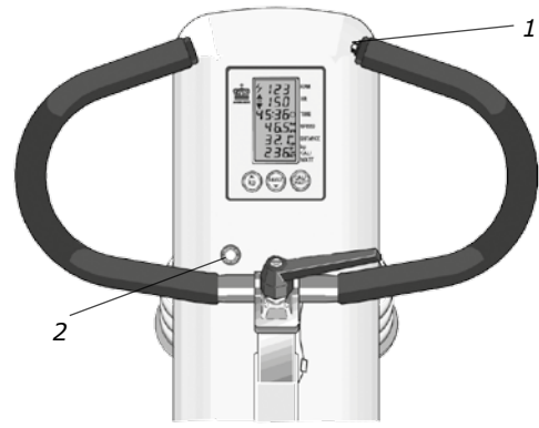
Fig: Workload adjustment 1) Release button, release basket 2) LED
